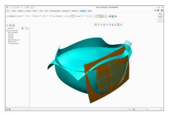
Curve and surface definition can also be generated manually with full control over the surface control mesh if desired.
