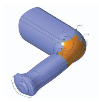
Advanced surfacing tools inside Creo ISDX allow for the creation of high quality surfaces when more than 4 boundaries exist.
