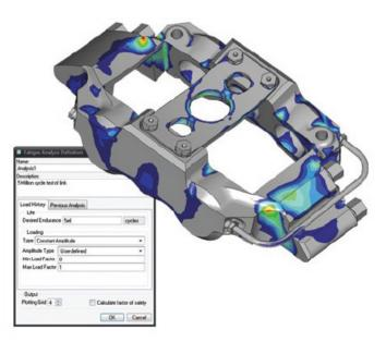
With PTC Creo Fatigue Advisor Extension, you can easily estimate the number of load cycles your model can sustain before failure.
