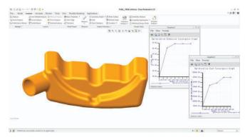
Creo BMX ensures your design meets its requirements. Here, we can ensure the designed tank will be able to hold the desired volume of fuel.
