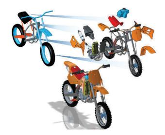
Creo AAX offers advanced assembly capabilities, such as skeleton models and data-sharing features, to support top-down design. Design criteria related to the assembly can easily be communicated to teams working concurrently on designs.
