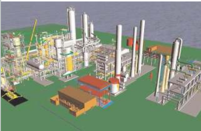
Factory site as 3D model – generated from scanner data
