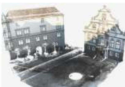
Colourmapping – 3D point cloud with RGB colour information
