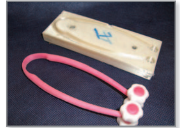
Akaishi used FDM to produce PPSF injection molds. It then produced several facial massagers, each from a different thermoplastic, for comparison.
