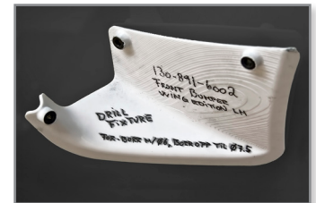
Front bumper drill fixture used to test the design.
